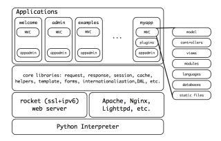
At the bottom we find the interpreter. Moving up we find the web server (rocket), the libraries, and the applications. Each application consists for its own MVC design (models, controllers, views, modules, languages, databases, and static files). Each application includes it own database administration code (appadmin). Every web2py instance ships with three applications: welcome (the scaffolding app), admin (the web based IDE), and examples (copy of website and examples).
